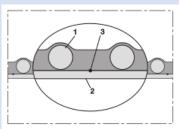
Antistatic polyurethane hose, extremely heavy, grounding wire
